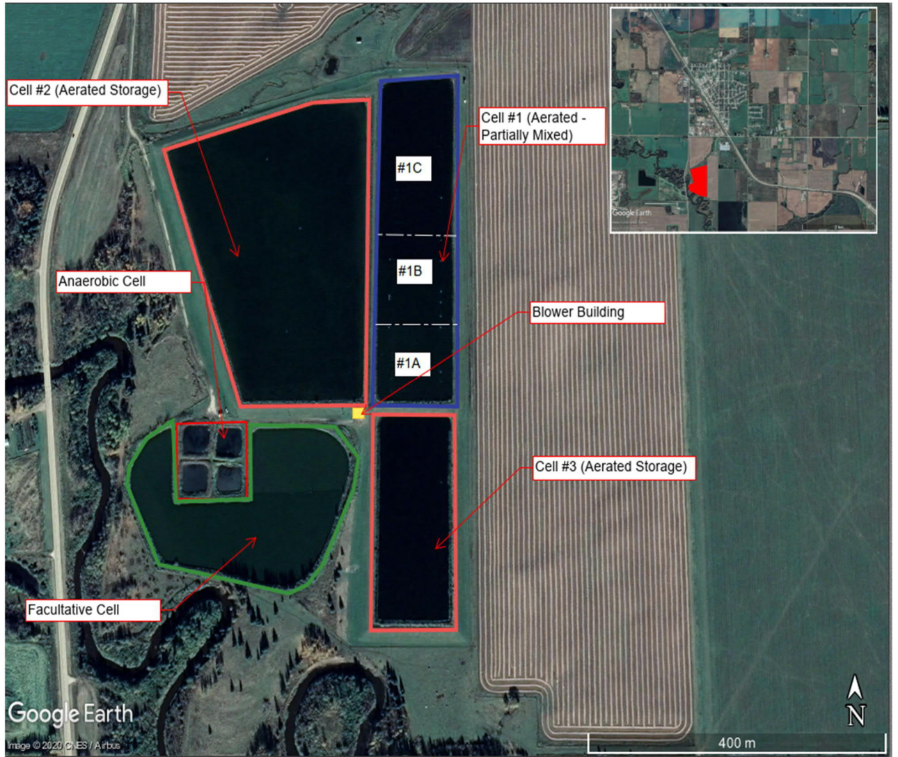
Figure 1-1 Town of Beaverlodge Wastewater Lagoon System Site Schematic
