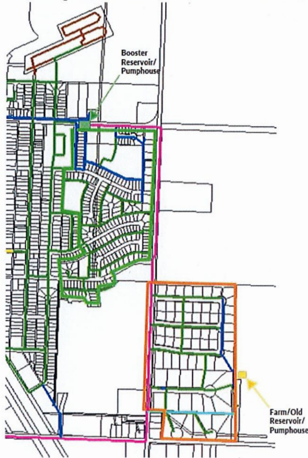
Figure 1-1 Beaverlodge Booster and Farm/Old Reservoir Distribution Zones
